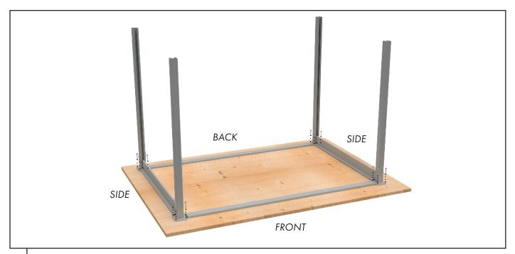
On top of a sacrificial board made from minimum 15mm thick structural timber, position posts using the provided guide slats to measure their location. Check measure the squareness of your layout as well as the outside distance between posts (which should match the defined width and depth of your enclosure). Adjust as necessary before screwing down posts into the sacrificial board.
