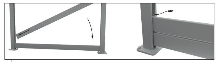
3 Build the enclosure SIDES by pivoting slats into position. Insert a spacer block above the first slat, followed by a slat, inserting into one post and levering the other side into the other post. Alternate between spacer blocks and slats. Do not install a spacer block on top of the final top slats. Use a rubber mallet if needed to ensure slats are fully pushed down in post.
