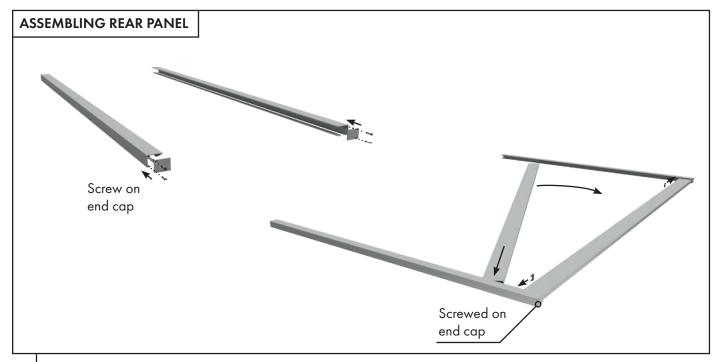
On a flat padded surface, position two back side frames. Screw fix on an end cap to each side frame and position capped ends of side frames same side. Install first slat directly onto end caps followed by spacer blocks (if using). Alternate between slats and spacers, and finish with a slat at other end.
