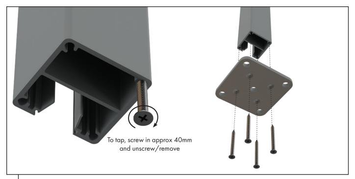
Using one of the supplied 12Gx50mm countersunk screws, tap all screw flutes in bottom of all 50x50mm friction fit posts. Attach base plates to posts using 4 x 12Gx50mm countersunk screws per post.
