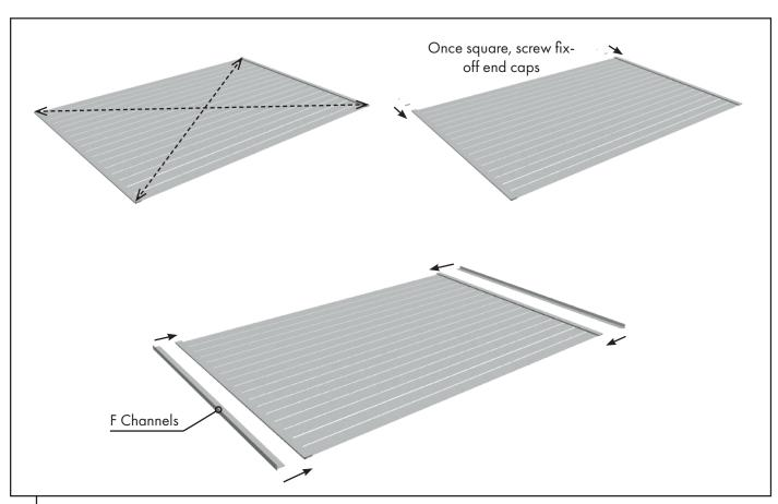
B Check measure closed back assembly is square, using a soft mallet to adjust and ensure all slats are positioned fully down and inside both side frames. Add end caps to open ends. Re-check squareness.
