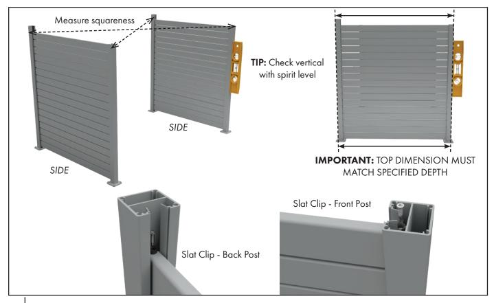
Once all slats are in position, check measure squareness of structure at bottom and top on both diagonals.
