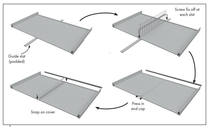
Re-use guide slat(s) positioning under the lid in the centre of the slats where centre support rail will be positioned. Ensure protection or padding is used between guide slat and lid.
