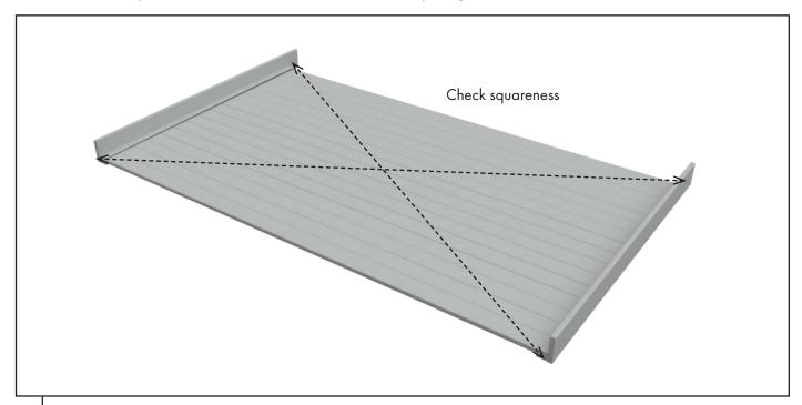
Check measure squareness of lid, measuring corner to corner. Adjust as required with a padded rubber mallet, taking care not to dent/damage any parts.
