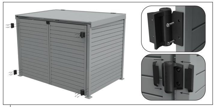
Attach 2 x hinges to each door with 3mm pilot holes and 4 x 10Gx16mm wafer head screws screws per hinge: 2 screws into holes at front of door and 2 screws going into the door through the side leg of the hinge. Equally space hinge from top and bottom at around the 3rd slat up/down or as desired.
