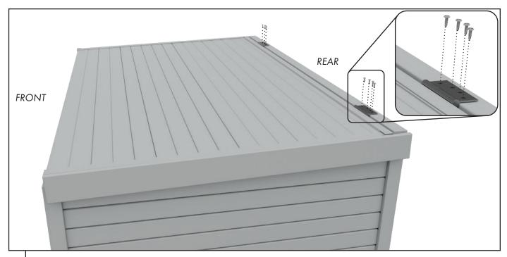
Using help as required, carefully lift lid into position and locate with hinge knuckle resting against top of capped 50x50mm profile. Drill 4 x 4mm pilot holes per hinge and screw off hinges into top surface of capped post with 4 x stainless steel 10Gx16mm wafer head screws.
