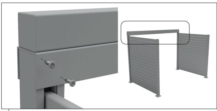
Flip over and position U Channel/Profile sub-assembly over the back posts of enclosure. Drill 2 x 3mm pilot holes on front side of channel into back posts and affix with 2 x 10Gx16mm wafer head screws on front side of each post.
