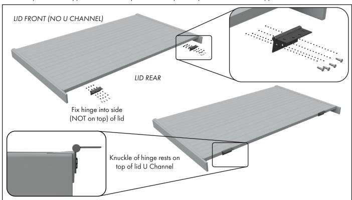
Carefully turn lid over. Position hinges onto U Channel on lid equally positioned from each end, approximately 100-250mm in from edges depending on enclosure width. Drill 4mm pilot holes for the hinges and screw off with 4 x stainless steel 10Gx16mm wafer head screws.
