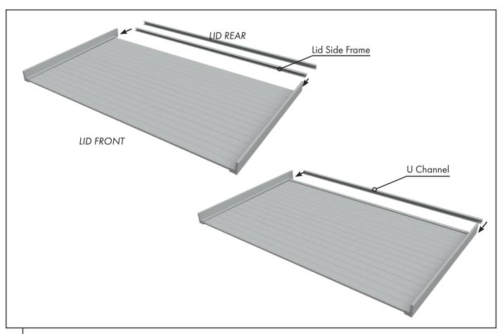
Add side frame to rear open end of lid assembly (i.e. end without end caps on side frames).
