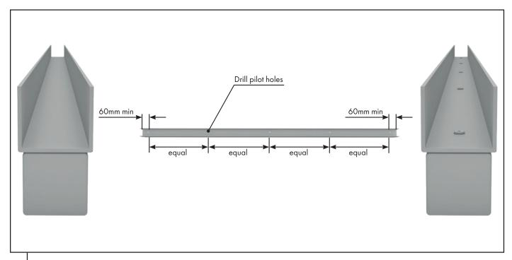
Position the U channel centrally on the capped 50x50mm profile. Measure 60mm in from each end and drill 5 x 3mm pilot holes equally spaced through U channel and first wall of post. Affix U channel to post with 5 x 10Gx16mm wafer head screws.
