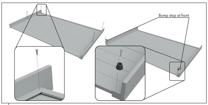
Drill 3mm pilot holes through side frames into slats: 1 x pilot hole at back slat (through U Channel), 2 in middle slat 1 at front slat. **NOTE:** Front hole uses bump stops - use as a guide to position bump stop close to the front edge of the lid.
