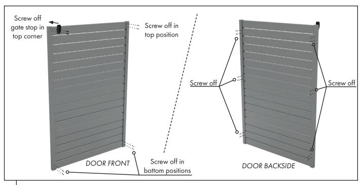
Screw off side frames to slats with 3mm pilot holes and secure with 10Gx16mm wafer head screws.
