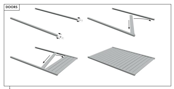
3 Screw fix end plates to 1 end of each door side frame.
