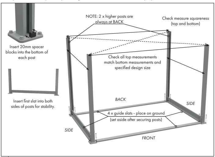
Insert 20mm spacers into the bottom of the side posts so that the spacers sit on top of the base plates. Then insert first slat into both sets of posts on top of 20mm spacers for stability.
