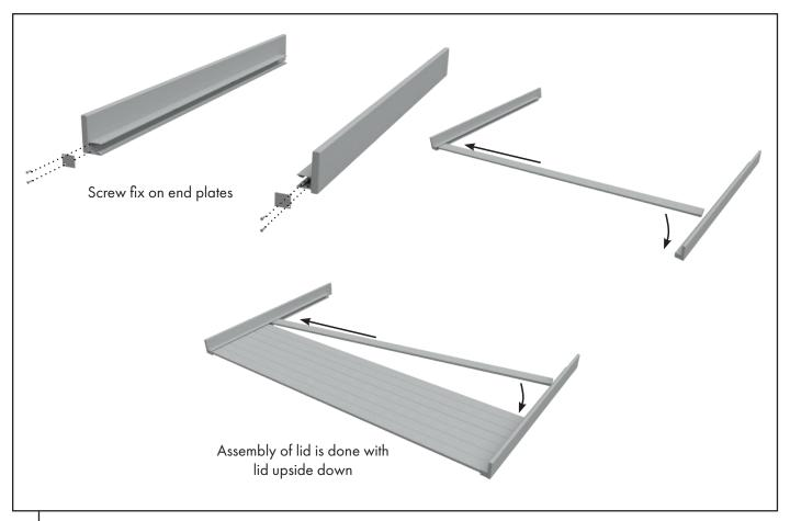
Lay left and right lid side frames on a flat padded surface with the side frames at the bottom and facing each other. The extended 90mm slat will face the back of the lid. Screw fix on end plates to the front of both side frames with 2 x countersunk screws ensuring end plates are added to the same side as laid out (see above).
